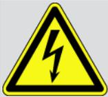
This symbol indicates dangerous electric voltage/high voltage.
